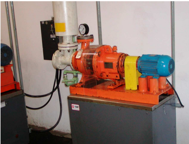
FIGURE 12 – PUMP SIMULATOR TEST RIG
