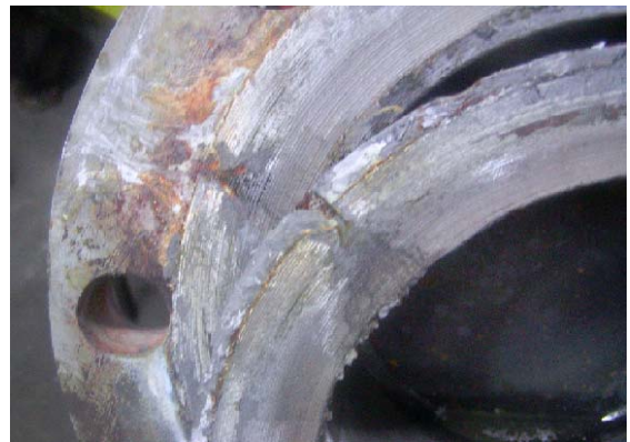
Figure 19 - Blowout of Style E
