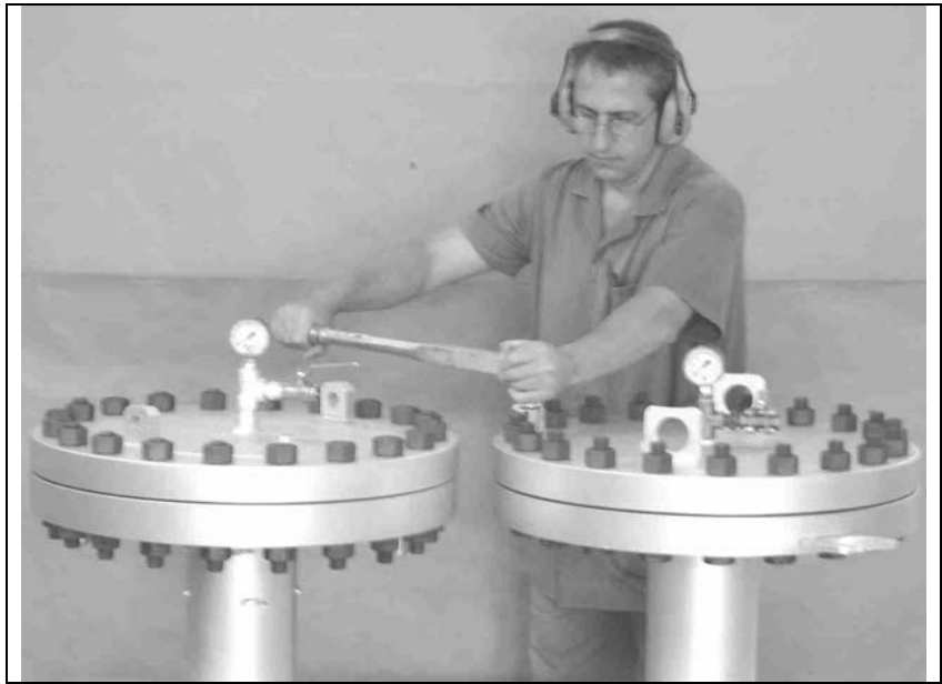
Figure 8 – Sealability test stands
