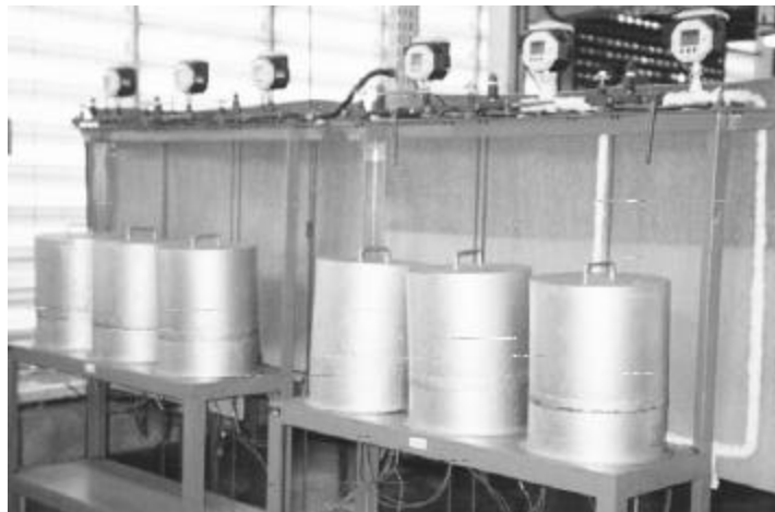
Fig.3: Class 150 and Class 300 test cells - insulated.
